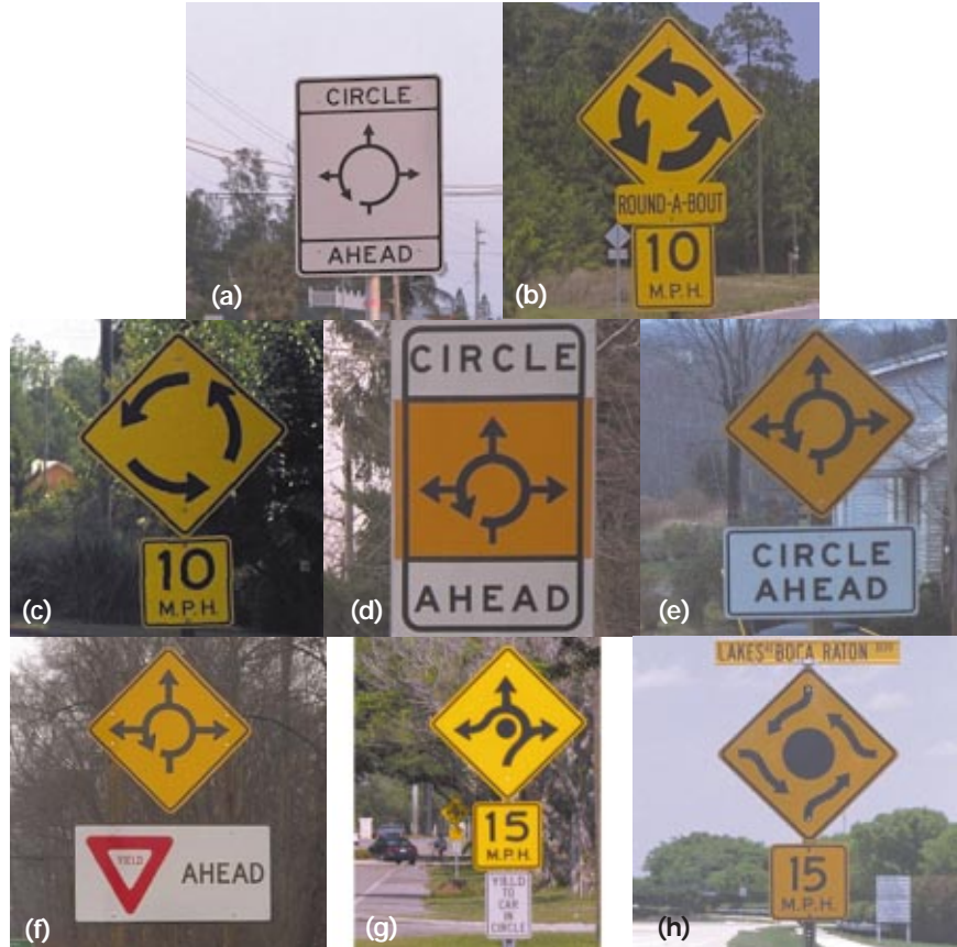
Exhibit C-3. Sample of existing Roundabout Ahead signs in United States.
